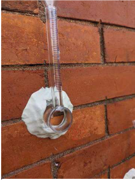
Rilem Test Tube – T-Joint
