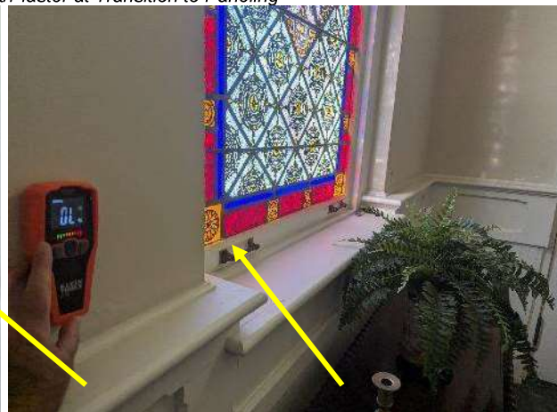
Elevated Moisture Content Adjacent Door & Adjacent Window
