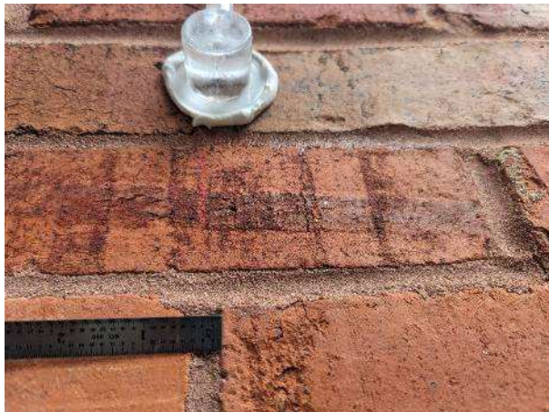
Rilem Test Tube – Head Joint
