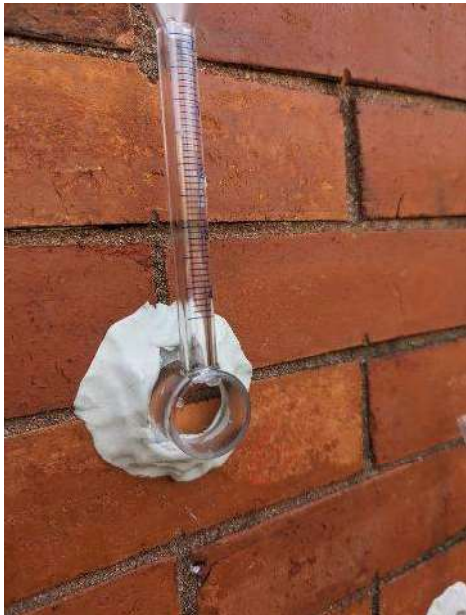
Rilem Test Tube – T-Joint Test #6
