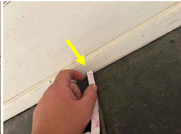
Water Detection Paper (Pink Color) Identifying Water Infiltration
