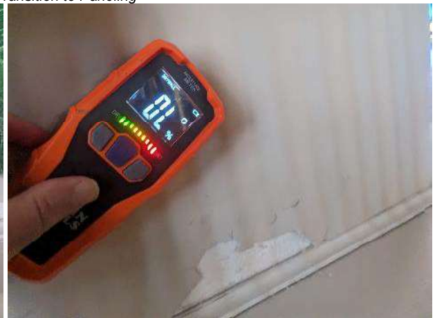
Elevated moisture readings in paint and plaster
