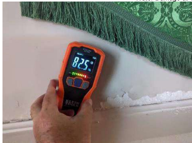
Elevated moisture readings in paint and plaster
