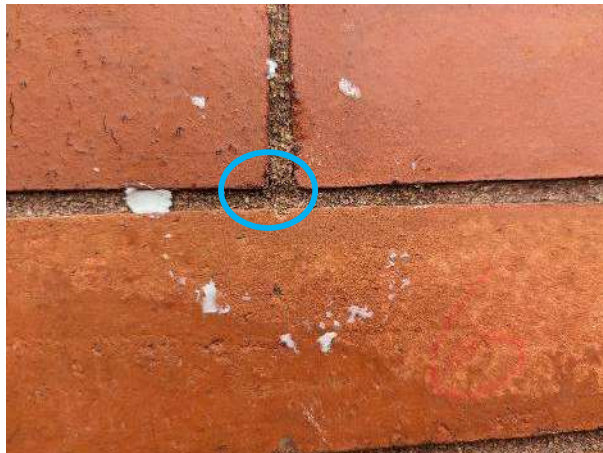
Rilem Test Tube – Test #6 – 4.5ml Absorbed in Less than 1-Minute with Small Void in Mortar Visible.
