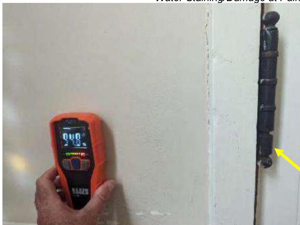
Elevated Moisture Content Adjacent Door & Adjacent Window
