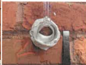
Rilem Test Tube - Bed Joint: Wetting / Absorption of Mortar during Testing
