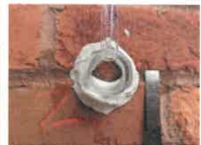
Rilem Test Tube - Bed Joint: Wetting / Absorption of Mortar during Testing
